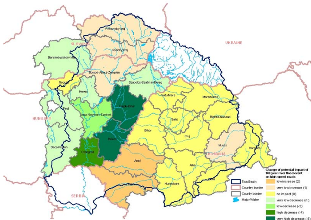
Map 6: Change of potential impact of 100 year river flood event on high speed roads
