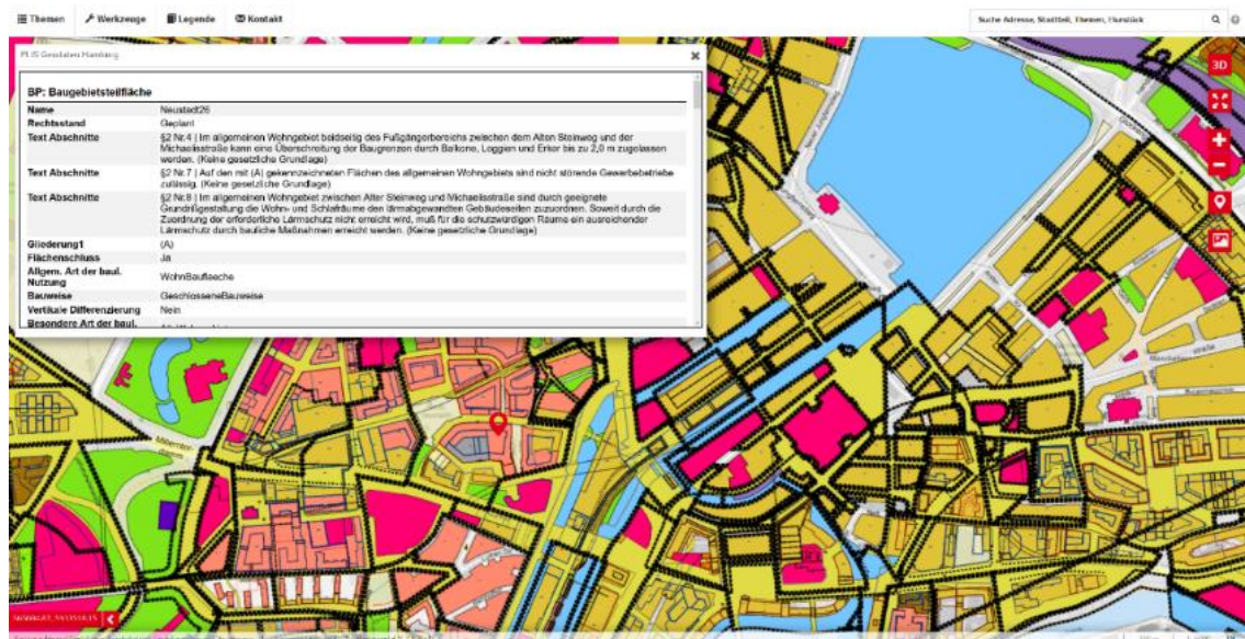
Figure 3.6 Full vector dataset of the land-use plans in Hamburg, showing the textual determinations for a specific plot (marked red)
